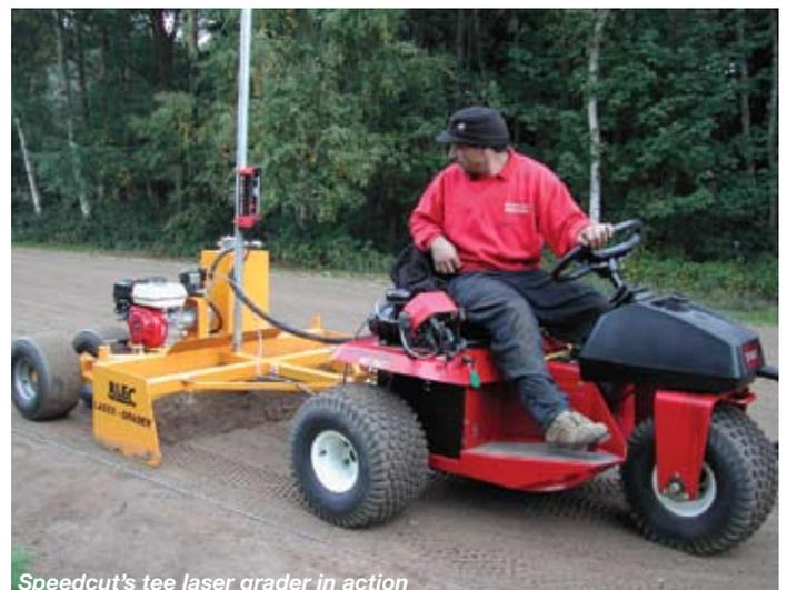
Speedcut's tee laser grader in action
